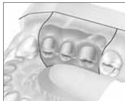
Figure 18. The metal framework is placed over the Fixed Abutments to evaluate fit.
