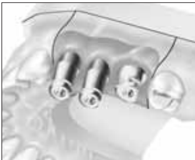
Figure 15. Impression Posts transfer the position of the patient's implants to a stone model.
